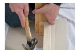
Optional – we used a shim to keep the  $2\times4''$ s in place when assembling the frame. As well, we applied wood glue before screwing in the jig holes. You could use clamps to secure instead of a shim.
